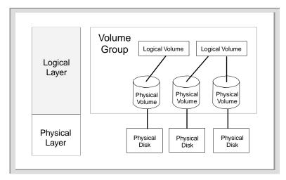
Each individual disk drive is logically represented by a physical volume (PV). Each physical volume consists of several partitions called physical partitions (PP). The physical partitions are grouped into something called a logical volume that contains logical partitions. The logical volume, in turn, belongs to a volume group. Logical volumes contain the file systems (like the Journaling File System or JFS).
