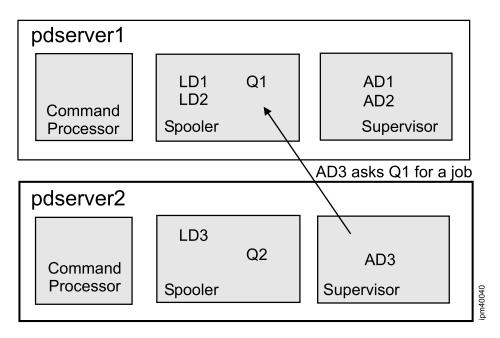
This is an example of a spooler part communicating with a supervisor part in a different pdserver. In this case, the queue associated with the actual destination sends a job to the actual destination for processing.
