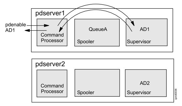
This example shows a command processor part communicating with a supervisor part in a different pdserver.
