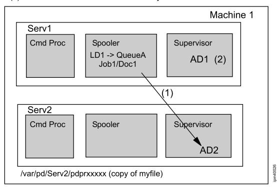
4. If the pdserver containing the actual destination is on a different machine than the command processor pdserver, the actual destination's pdserver communicates with the command processor pdserver to pull the file over to its machine.
