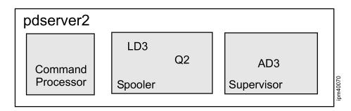
Here is an example of a supervisor part communicating with a command processor part in a different paserver. In this case, the actual destination requests the print file for the job from the command processor that processed the original **pdpr** request.
