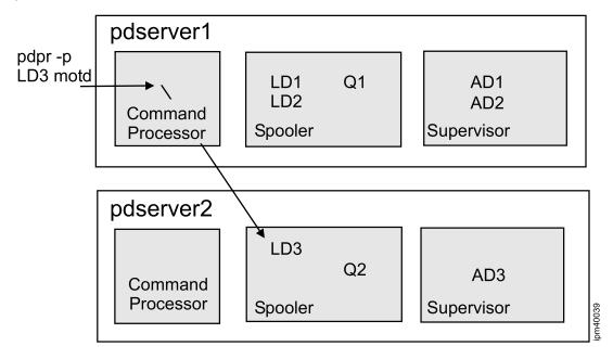
Here is an example of a supervisor part communicating with a spooler part in a different pdserver. In this case, an actual destination requests that its associated queue send it a job.
