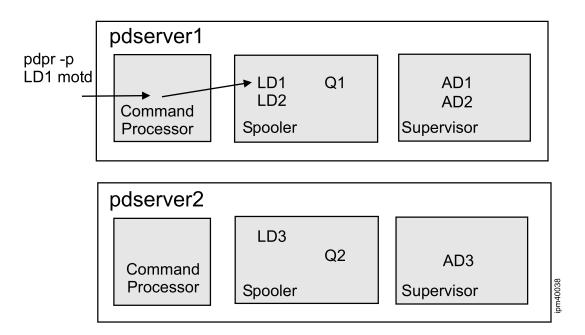
This example shows a command processor part communicating with a spooler part in a different pdserver.
