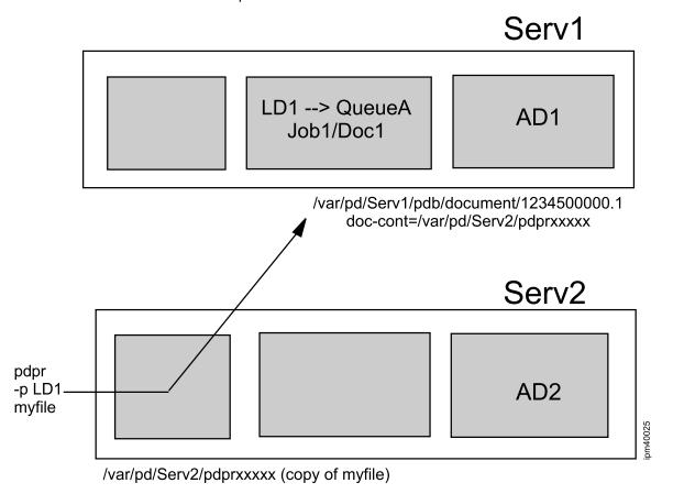
3. The job is scheduled and sent to an actual destination. The actual destination might be in a pdserver on the same machine or a different machine than the command processor pdserver. If the pdserver containing the actual destination is on the same machine as the command processor pdserver, the file is accessed directly by the actual destination.
