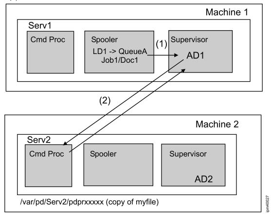
Files are "pulled" from one server to another using a socket. The command processor pdserver must be running for a file to be "pulled". When a file is "pulled", the actual destination stores it in its pdb directory. The "pulled" file is removed from the actual destination's server's pdb directory when the actual destination finishes processing the job, that is, it is completed or canceled.
