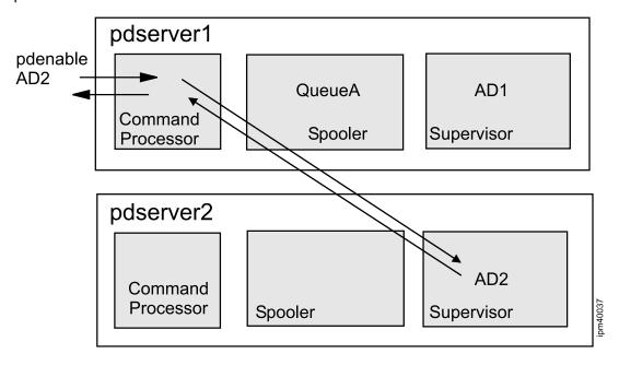
Here is an example of a command processor part communicating with a spooler part in the same pdserver.
