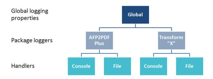
The logging properties file configures the operation of the AFP2PDF Plus logging facility. It consists of these three sections:
