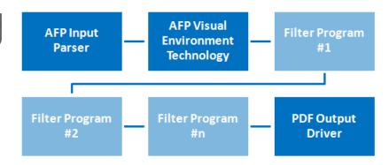
The AFP Input Parser works with AVE to run AFP filter programs. AFP filter programs are small JAVA programs, designed to do one thing and do it well. AFP filter programs can perform such operations as redacting text, deleting blank pages, or creating watermarks. Everything works together in a stream environment for optimum performance. Data is streamed from one program to the next and then sent to the PDF Output Driver.
