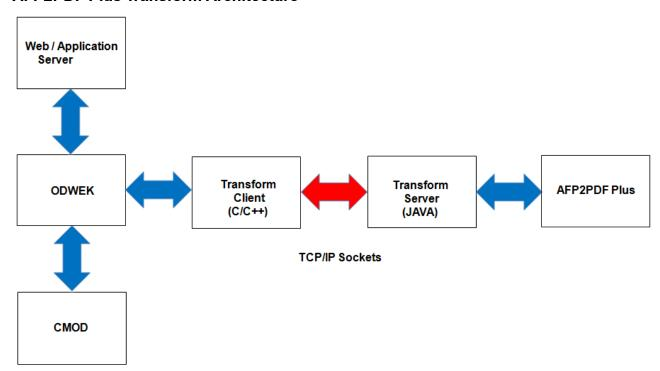
Since the new AFP2PDF Plus for JAVA Transform is designed to integrate with existing AFP2PDF installations, it has both client and server functions.
